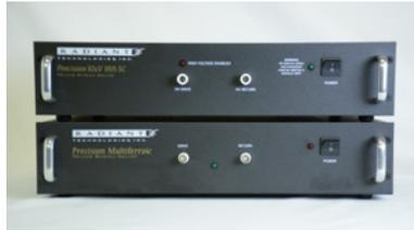
The Precision Multiferroic tester allows 30kHz measurements using the 200V internal amplifier and 50kHz measurements using the 100V internal amplifier.
